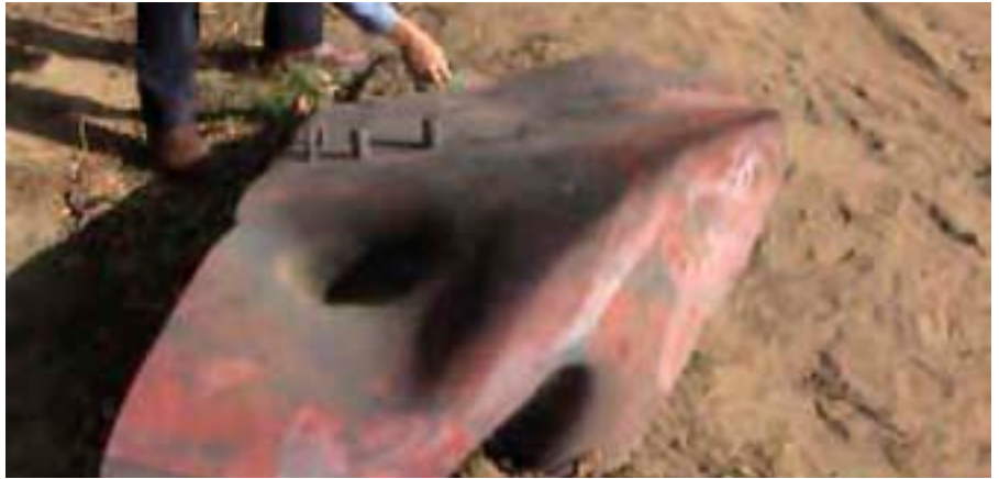
The photos by Ettore Contestabile from TNT Equivalency of Firework Shells: an insight into the Carmel Explosion, show the door (above) and the roof of the container; both hurled hundreds of metres.
