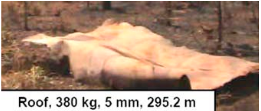
The photos by Ettore Contestabile from TNT Equivalency of Firework Shells: an insight into the Carmel Explosion, show the door (above) and the roof of the container; both hurled hundreds of metres.
